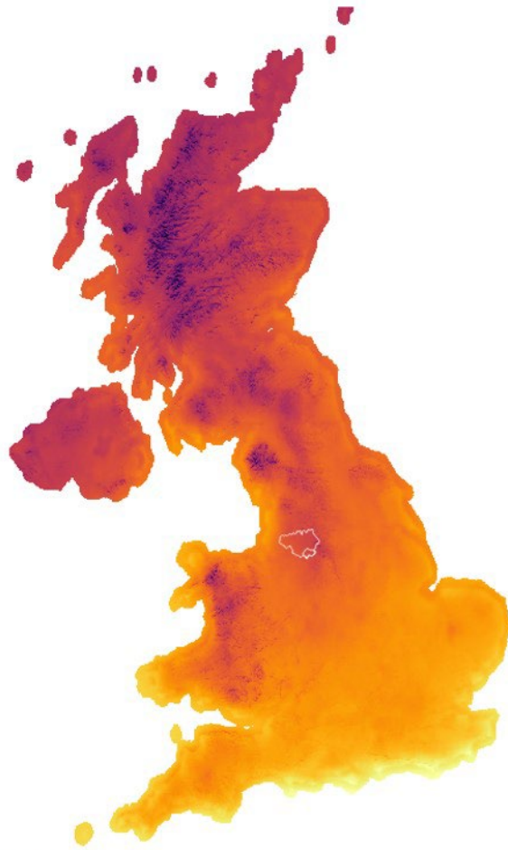
Figure 3.17: Predicted output from solar photovoltaics across the UK. The outlines of Greater Manchester and Stockport are shown in white.
